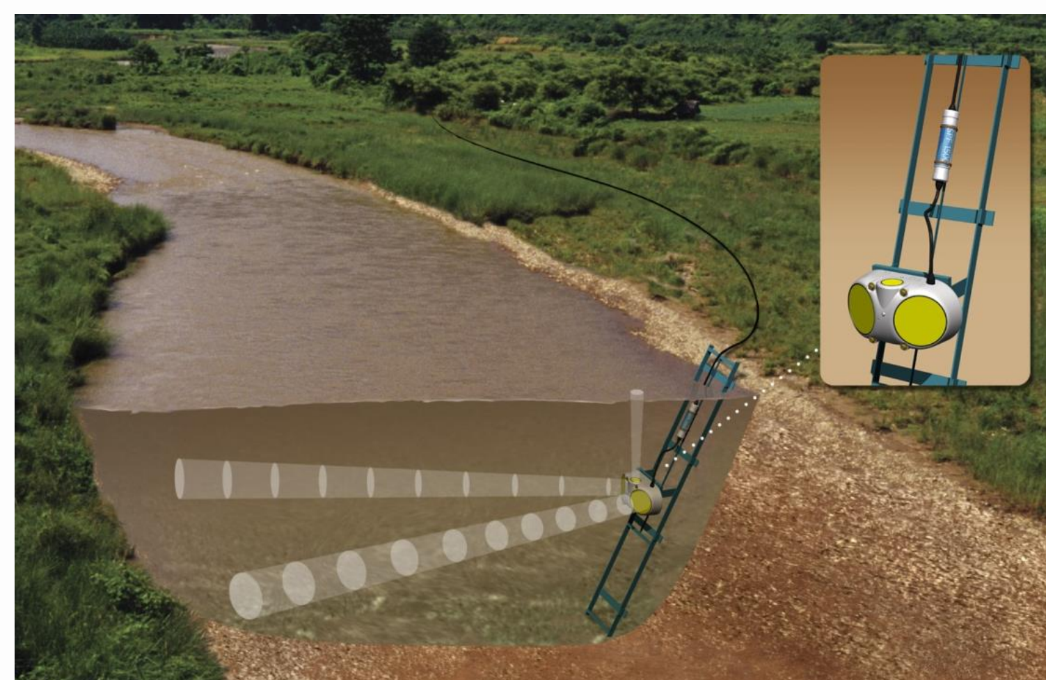
Figure 2: SonTek-SL measurement principle is based on two acoustic beams each slanted at 25° off the instrument axis. The system measures velocity in a horizontal profile that is divided into multiple cells based on the user configuration.
