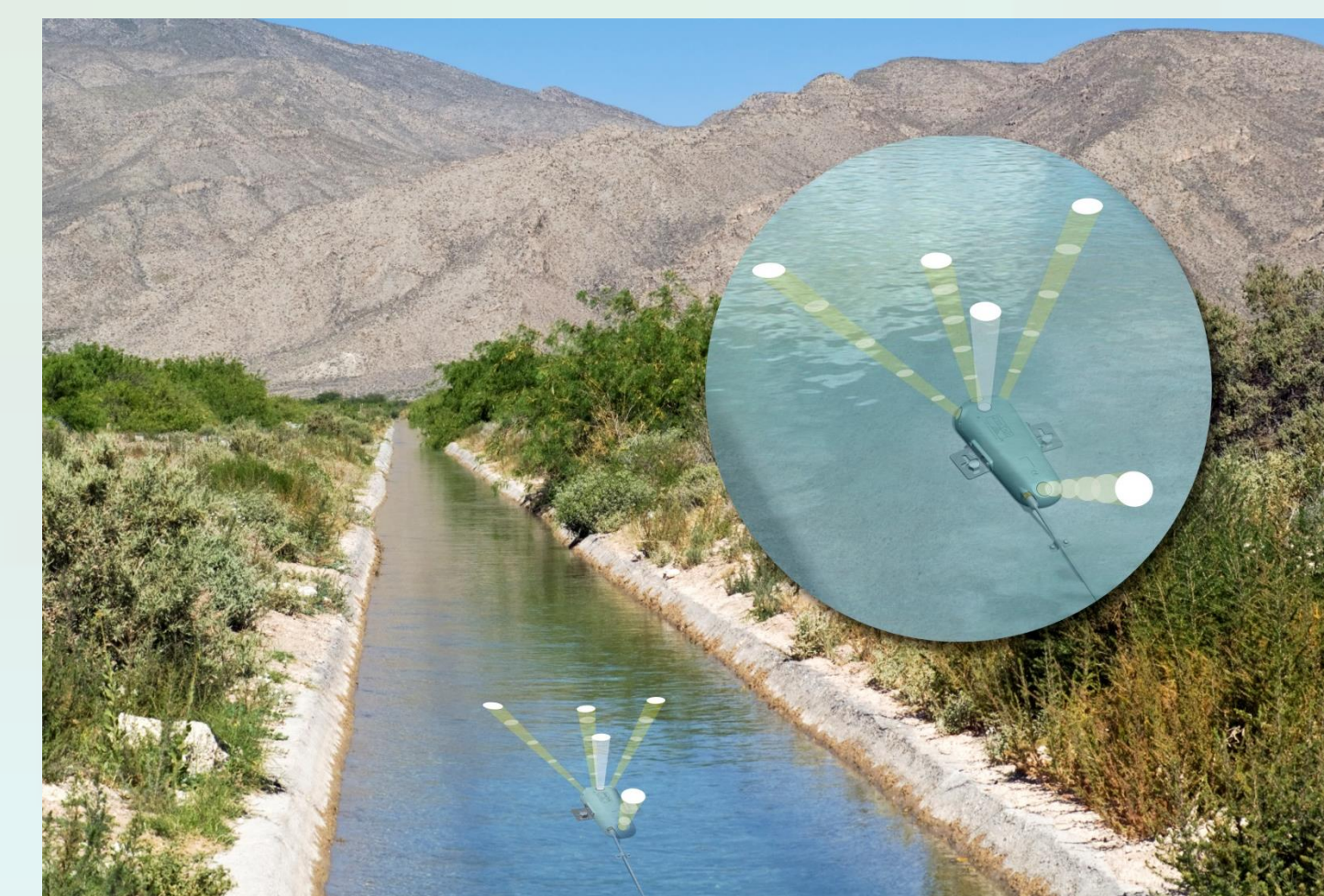
Figure 3: SonTek-IQ measurement principle is based on upstream and downstream acoustic beams along the axis each slanted at 25° off the vertical and two skew beams. The system makes use of SmartPulseHD that adapts the profiling technique, cell size and number of cells based on the flow conditions and water depth.
