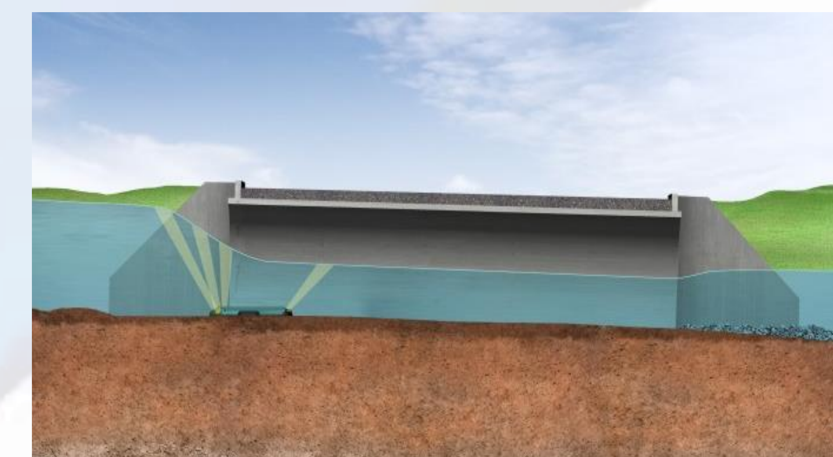
Figure 6: Supercritical flow conditions or multiple flow regimes within the affective measurement volume of the instrument can significantly impact the ADVM measurements and it is advised that these situations be avoided as far as possible.
